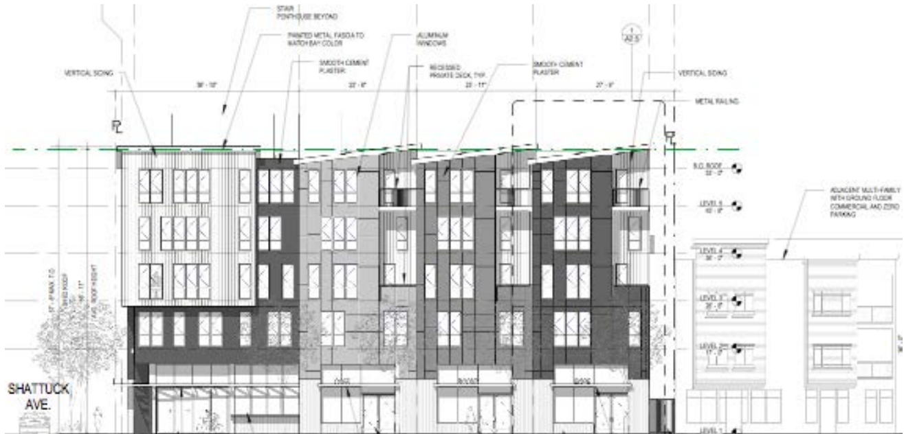
Figure 3a: North Elevation at Ashby Avenue (From January 30th, 2018) (For scaled plans see Attachment 2)
