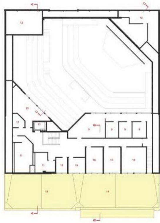
SECOND FLOOR 0 4 8 16 Preserved (Existing) 1. Entrance 5. Stage 9. Office 13. Elevator 2. Lobby / Performance Lounge 6. Green Room 10. Classroom 14. Roof 3. Ticket / Reception 7. Performer's Room 11. Restroom 15. Sound Position 4. Auditorium 8. Refreshments 12. Service / Storage 16. Service Corridor
