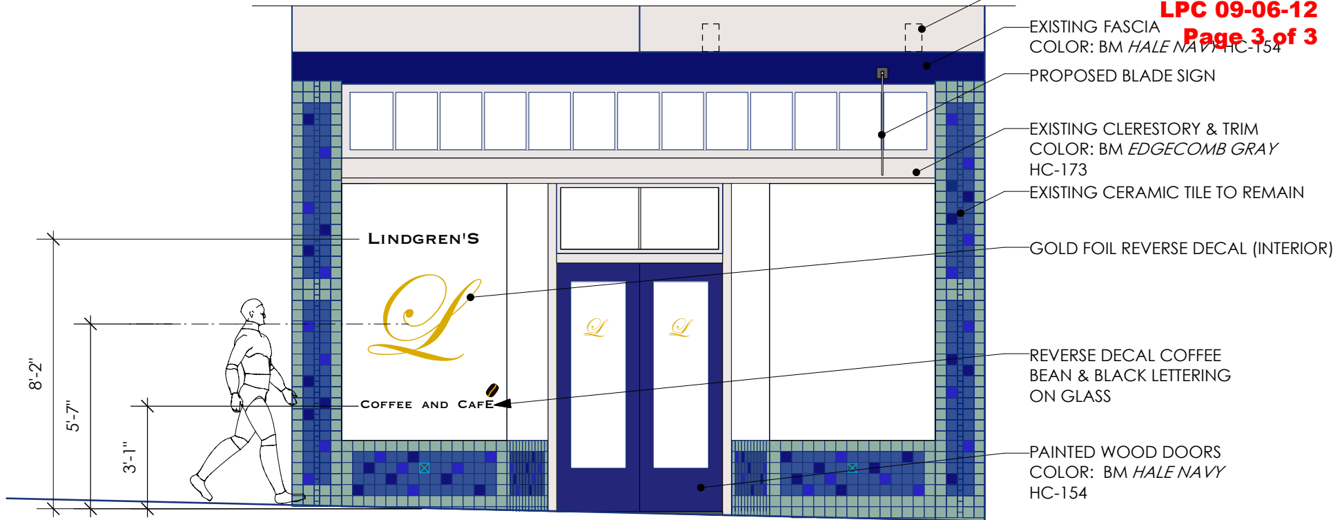
FRONT ELEVATION & SIGNAGE 1/4" = 1'-0"
