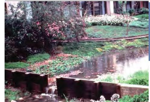
**Figure g.7. Landscaped Swales.** Swales gather and convey rainwater. Small “check dams” can be used to hold water in small ponds and release it slowly.
