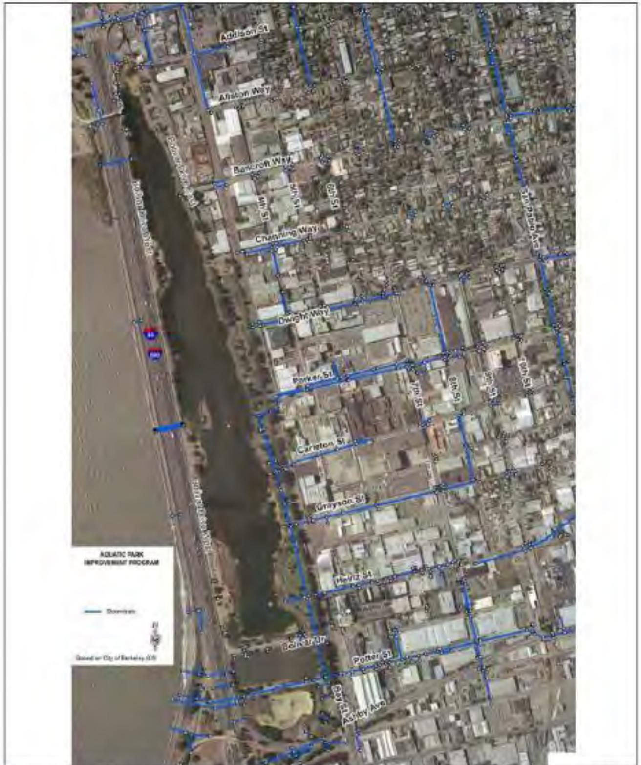
**ATKINS** **FIGURE 4.3-5** Aquatic Park Storm Drain Pipe Network Source: APP Figure 31, March 2011
