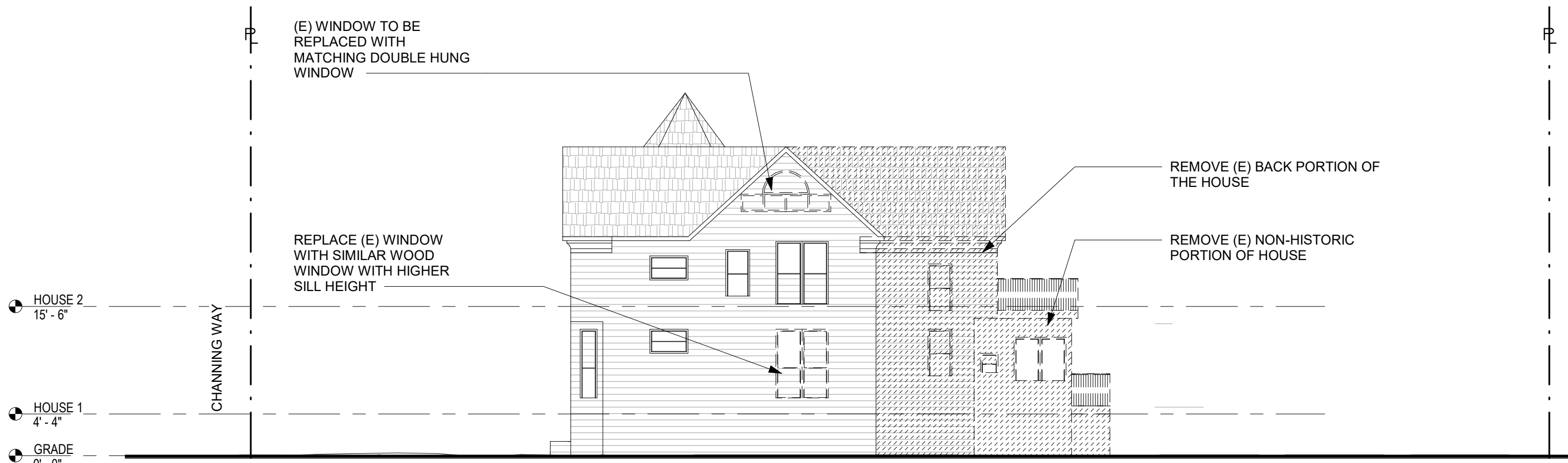
2 Existing/Demo West Elevation 3/32" = 1'-0"
