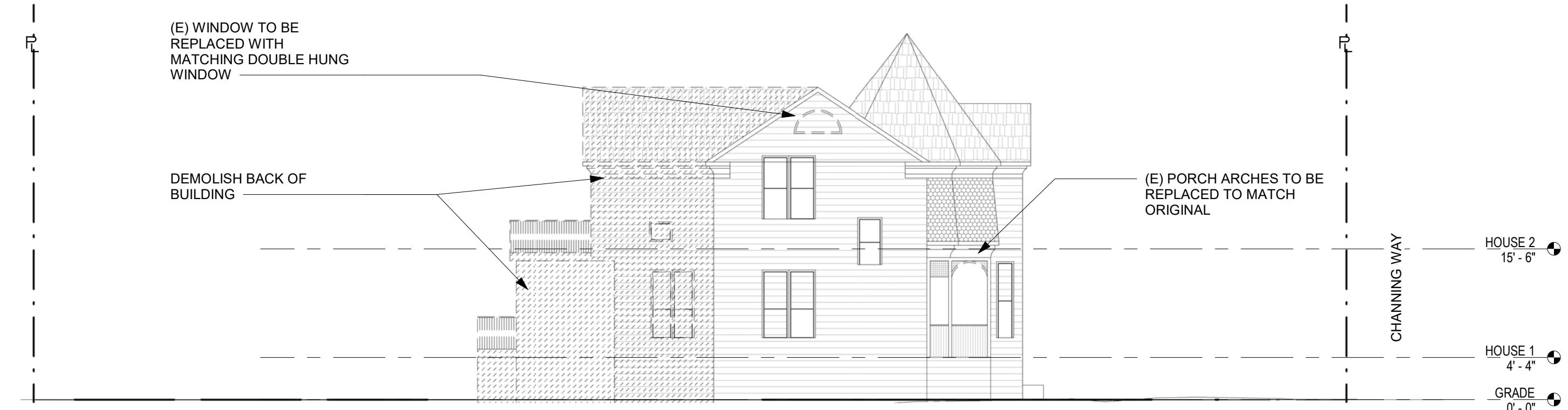
2 Existing/Demo East Elevation 3/32" = 1'-0"
