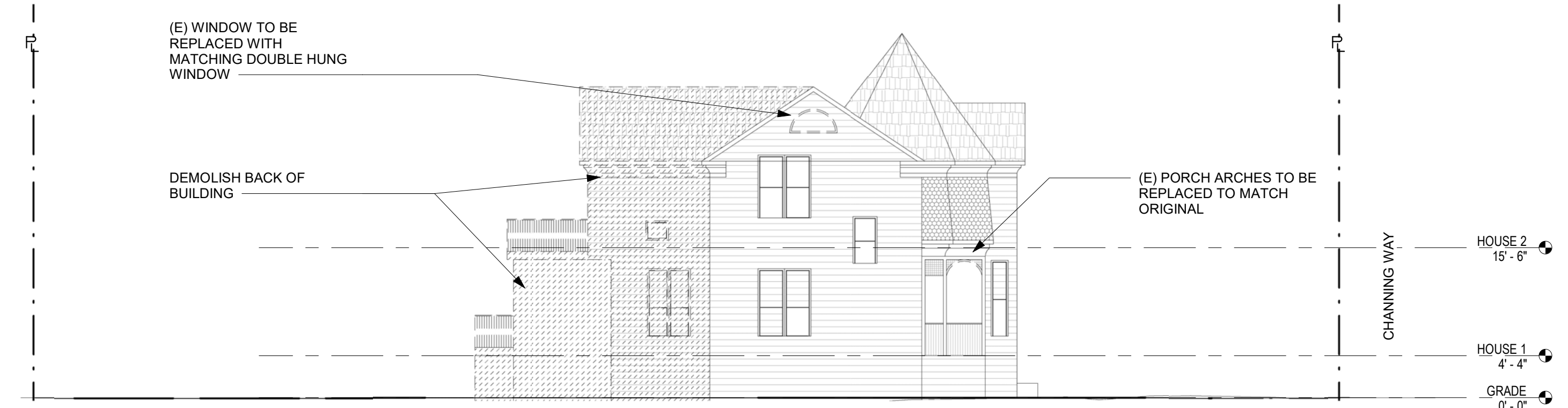
2 Existing/Demo East Elevation 3/32" = 1'-0"
