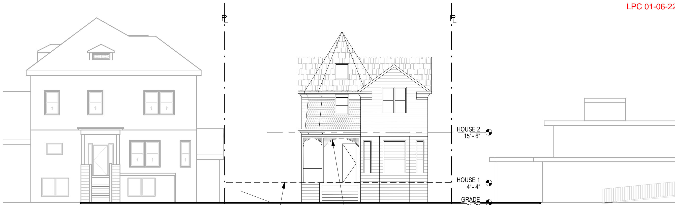
1 Existing/Demo North Elevation 3/32" = 1'-0"
