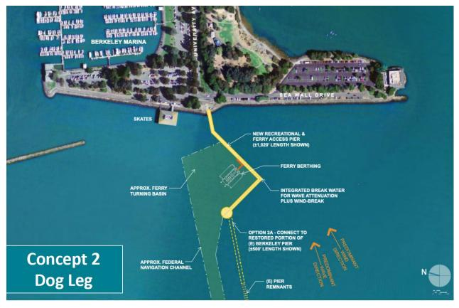
Figure 3-27 Concept 2 – Dog Leg Configuration
