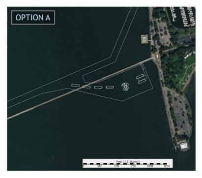
Figure 3-19 2018 Option A ferry terminal concept, located on south side of existing pier alignment
