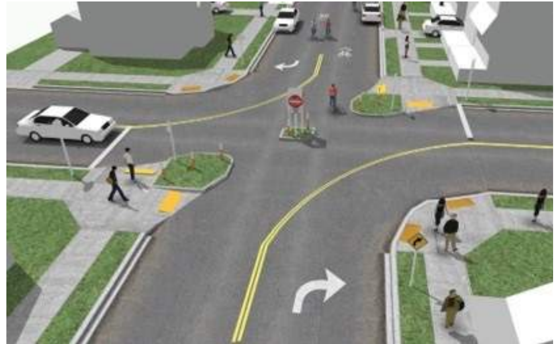
Diagonal Traffic Diverter
