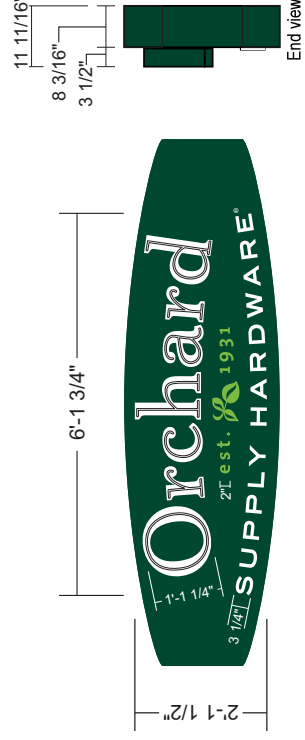
D TRADEMARK SKATEBOARD SPECIFICATIONS Scale: 1/2" = 1'-0" Manufacture and install one (1) trademark skateboard sign.
