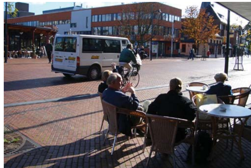
Figure e.8. Mixing Modes. Plaza-like features can be used to pedestrianize spaces while also allowing bicycles and motor vehicles. Motorists are presented with conditions that cause them to slow and yield as needed.
