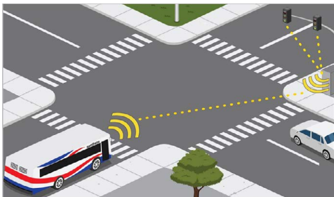
Figure 3.22. Transit Signal Priority Diagram. (Source: SamTrans)
