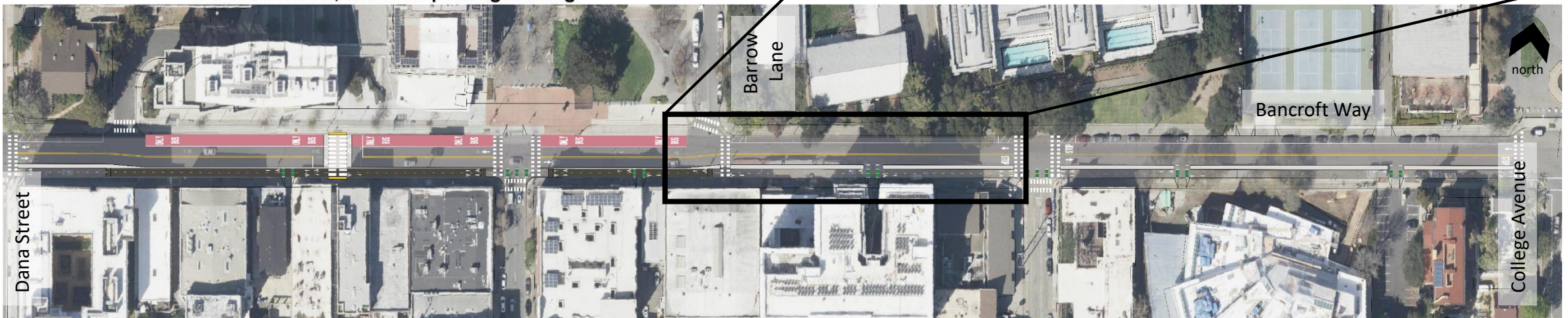
BANCROFT WAY - COLLEGE TO DANA (FACING WEST) Option Three: Two-way bikeway on south side, two-way vehicular traffic, curbside parking/loading
