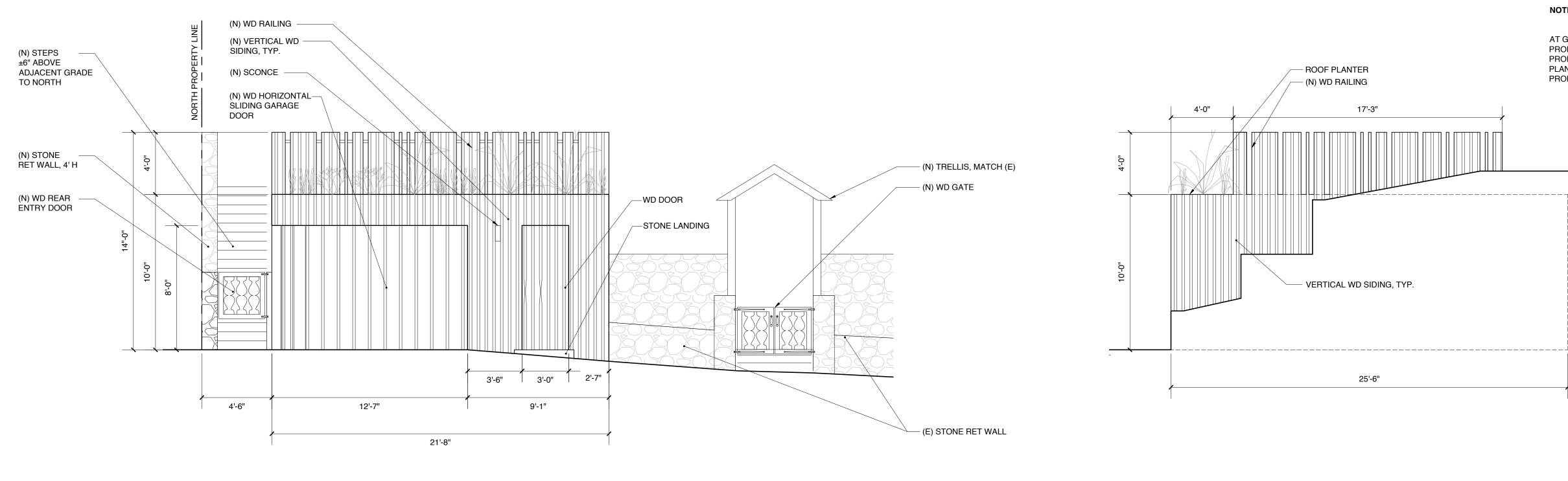
1: (N) WEST ELEVATION GARAGE 0 1' 2'  $\frac{1}{8}$ " = 1'-0" 2: (N) SOUTH ELEVATION GARAGE 0 1' 2'
