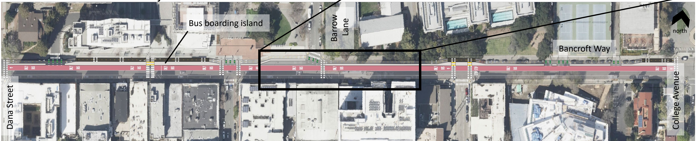
BANCROFT WAY - COLLEGE TO DANA (FACING WEST) Option Two: Two-way bikeway on north side Bus only lane on north side
