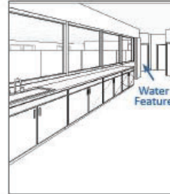
Security glazing allows staff to view the stabilization room through two-way windows (clients cannot see into the office) for monitoring and observation.
