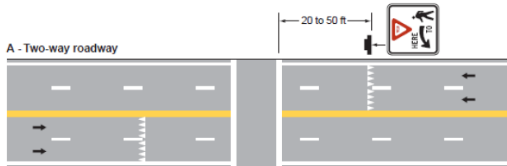
Figure 3B-17. Examples of Yield Lines at Unsignalized Midblock Crosswalks
