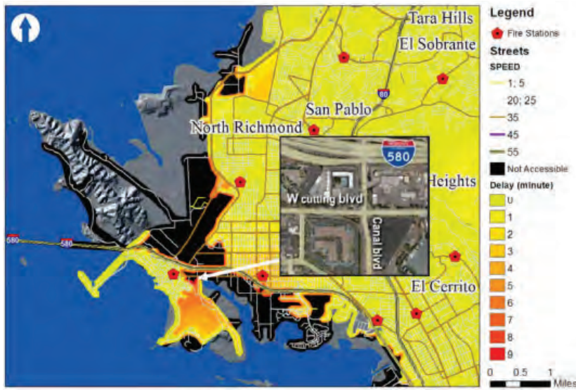
Delay in emergency response due to inundation of transportation network for Richmond, CA. Forcing scenario is 1.4 meters of sea level rise and a 100-year storm event. Areas shaded black are inaccessible due to the depth of inundation. Source: From Biging et al. 2012.
