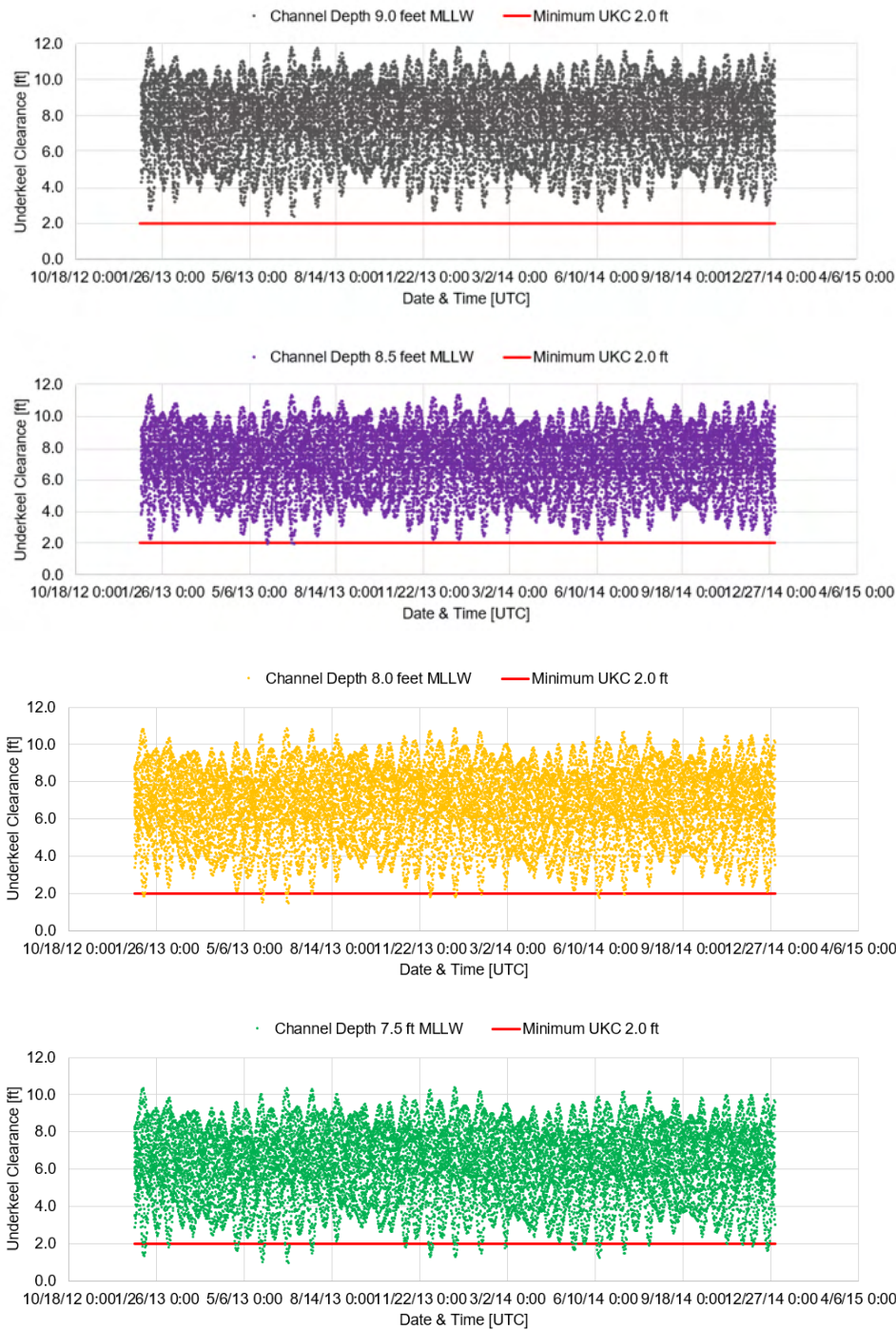
Figure 11: Underkeel clearances for channel depths between 9.0 feet MLLW (top) and 7.5 feet MLLW (bottom)
