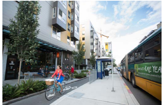
Figure 3.19. Bus Boarding Island. (Source: Green Lane Project)
