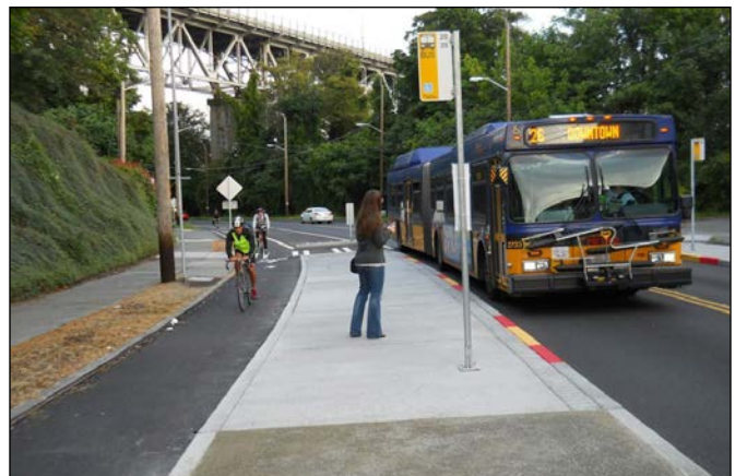
Figure 3.2. Bus Boarding Island on Dexter Ave, Seattle, Washington. (Source: NACTO)
