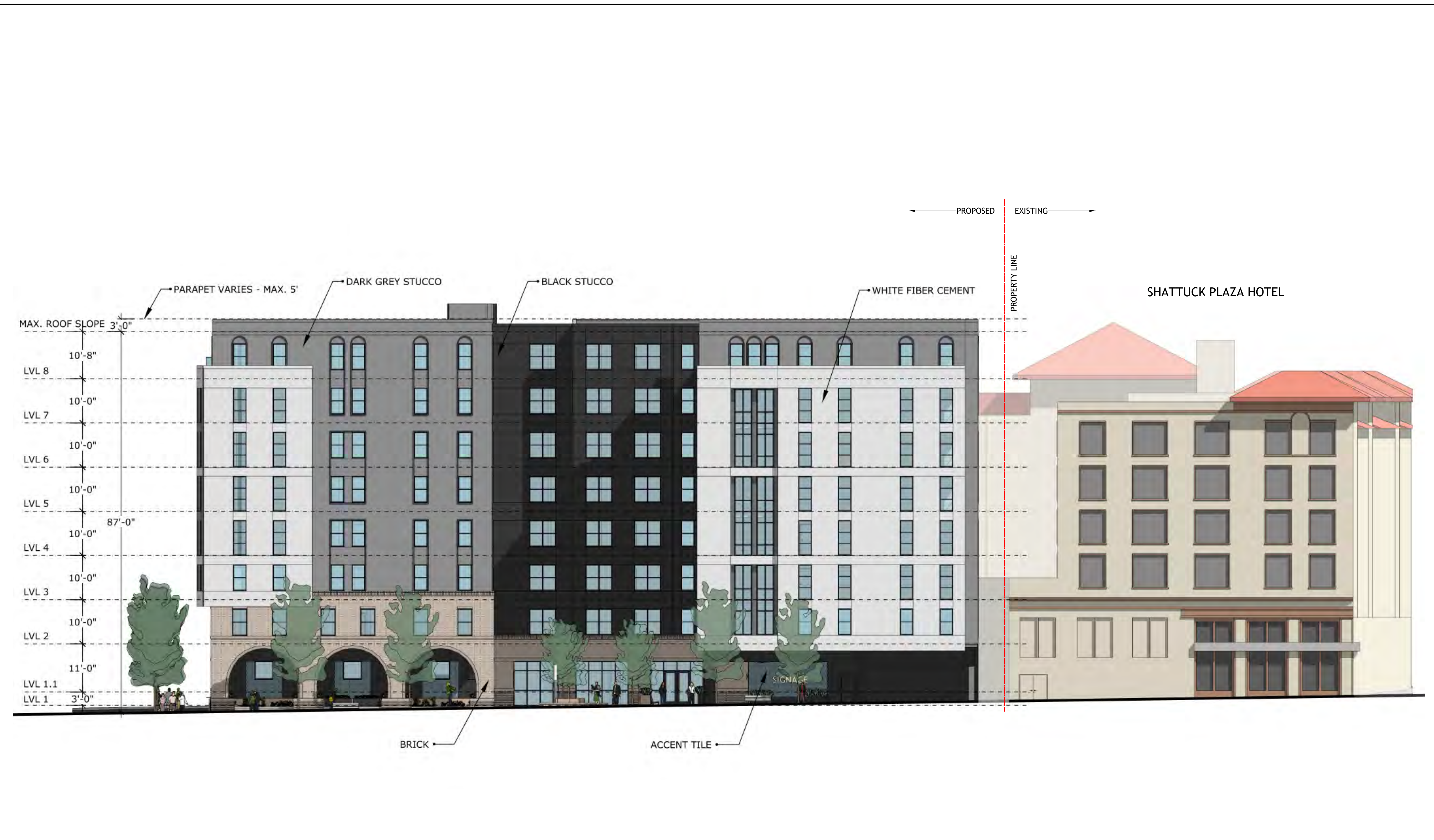
1 SOUTH ELEVATION - KITTREDGE ST A3-002 3/32" = 1'-0"
