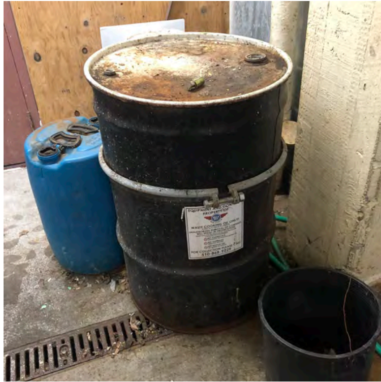
Photograph 7: Empty drum and anti-corrosion agent without secondary containment.
