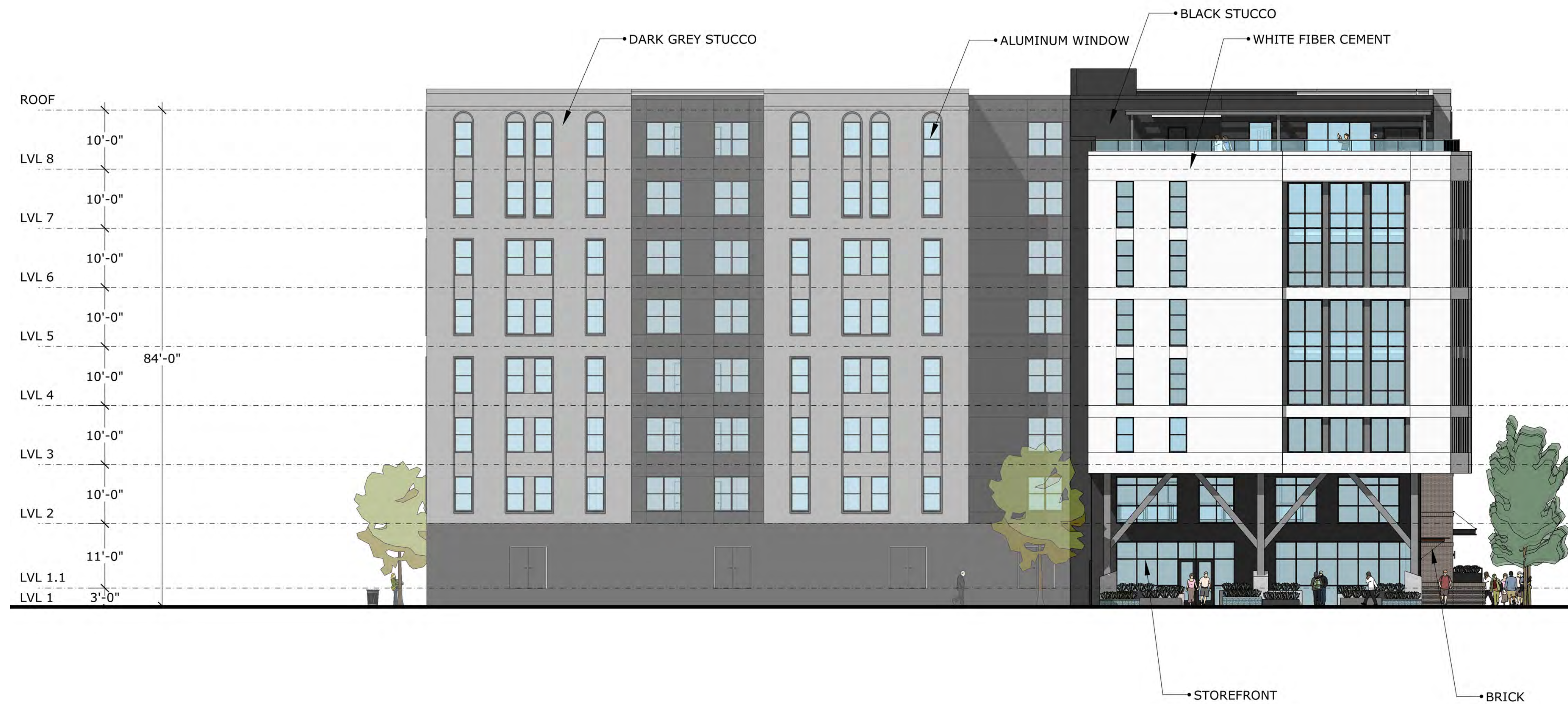
1 NORTH ELEVATION - ALLSTON WAY A3-003 3/32" = 1'-0"
