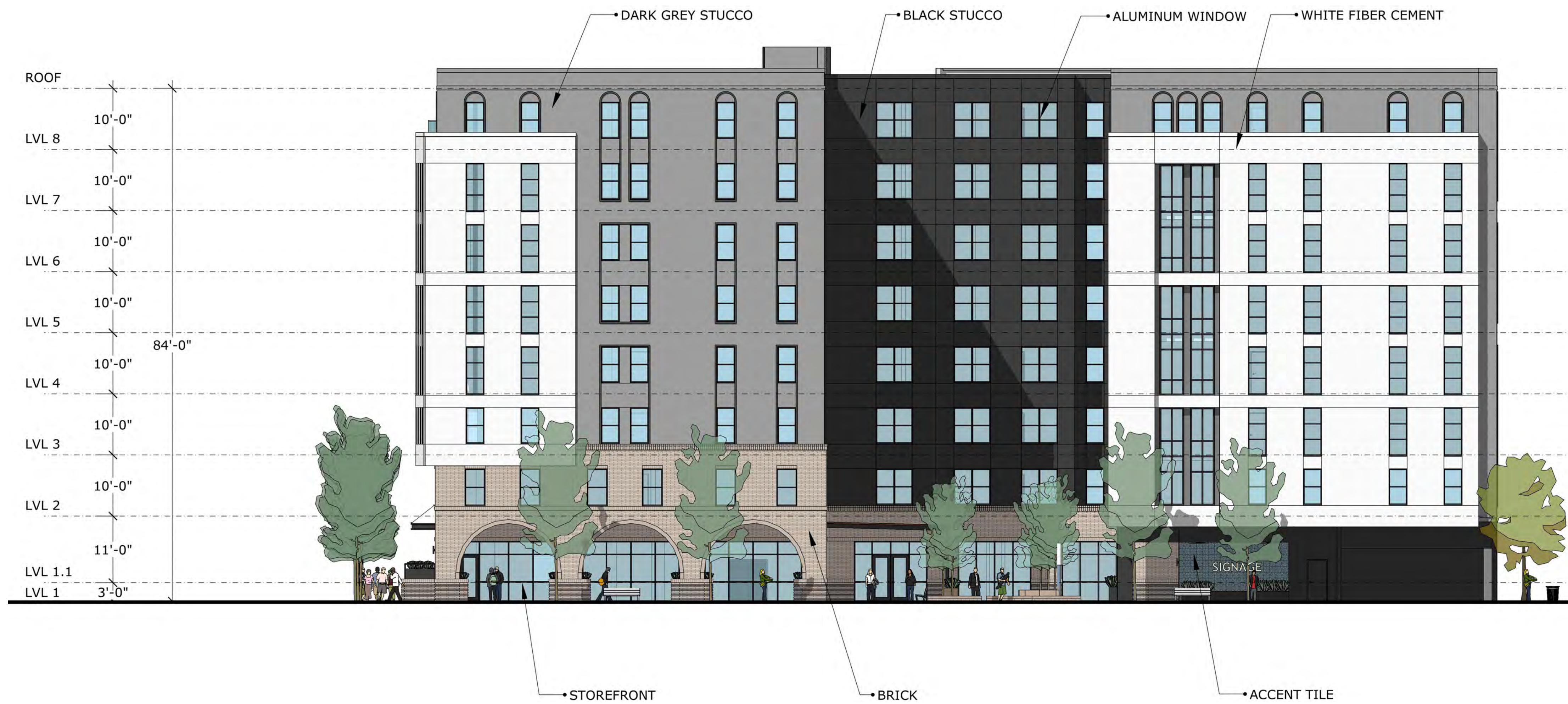
1 SOUTH ELEVATION - KITTREDGE ST A3-002 3/32" = 1'-0"
