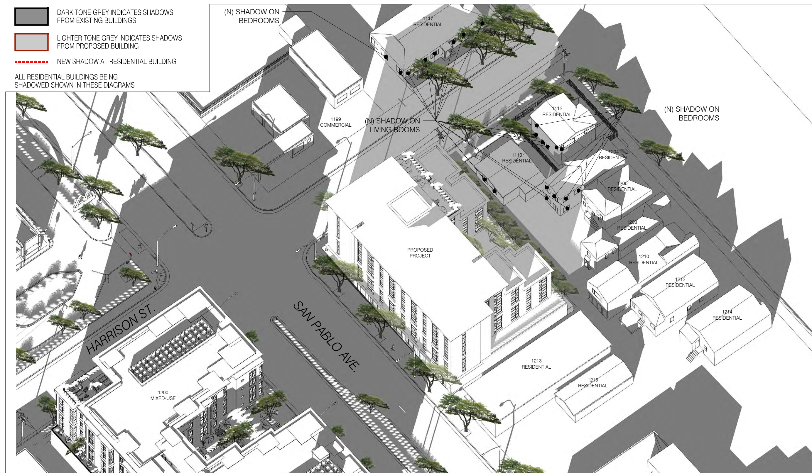
4 SHADOW STUDY AXONOMETRIC - DEC 21: 2-HRS AFTER SUNRISE NTS
