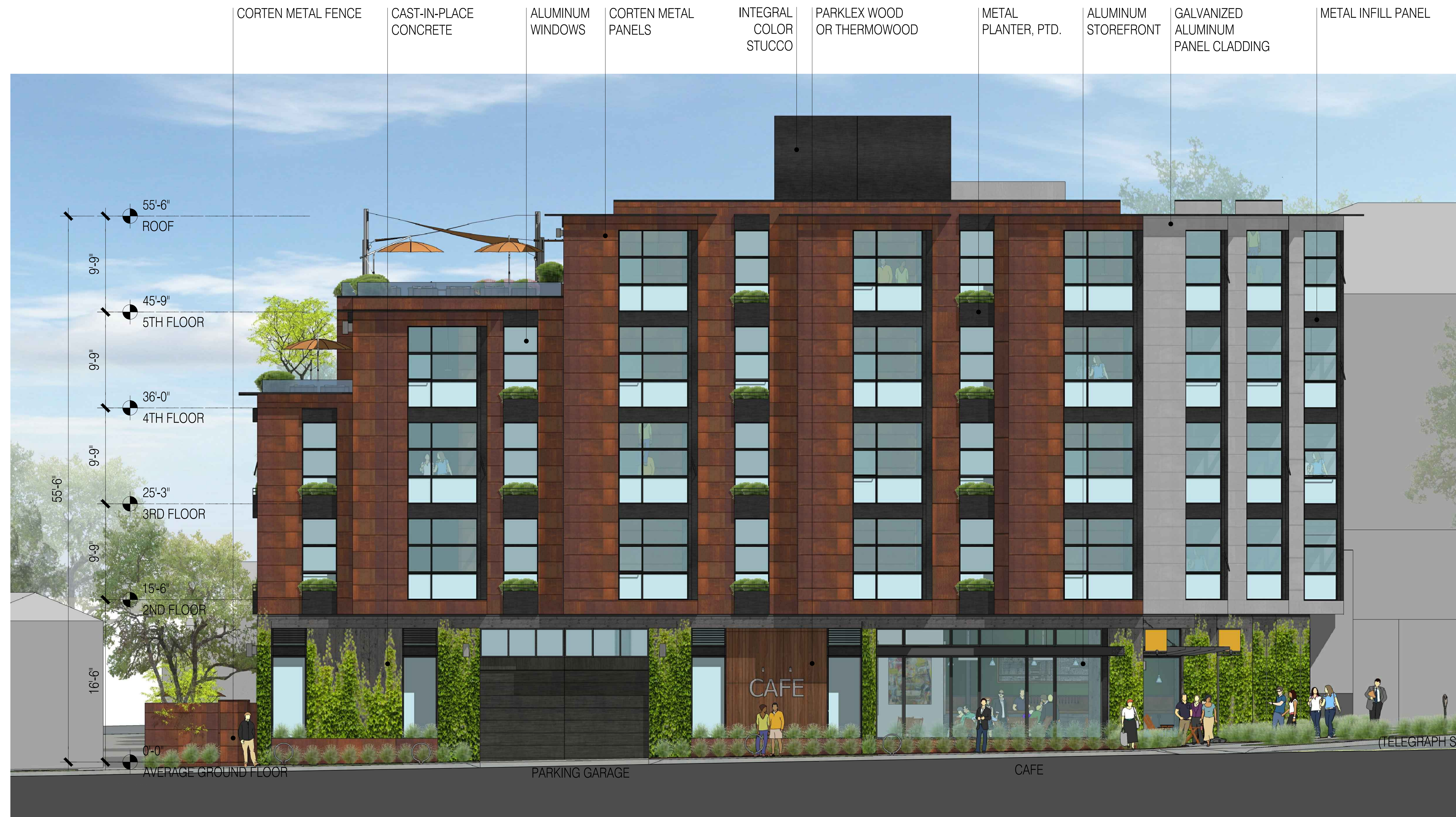
1 SOUTH ELEVATION 1/16" = 1'-0" @ 11X17 1/8" = 1'-0" @ 24X36
