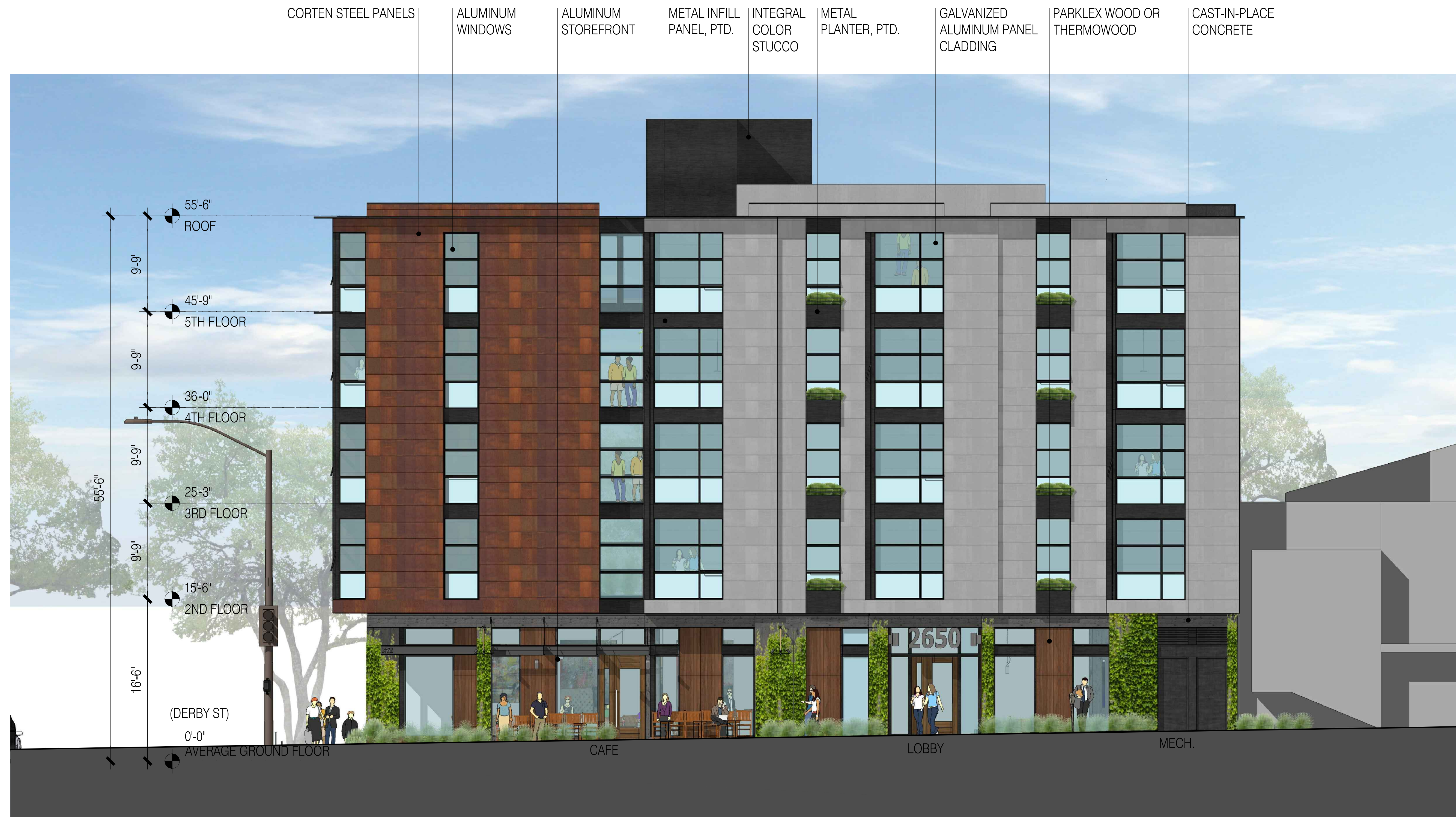
1 EAST ELEVATION 1/16" = 1'-0" @ 11X17 1/8" = 1'-0" @ 24X36
