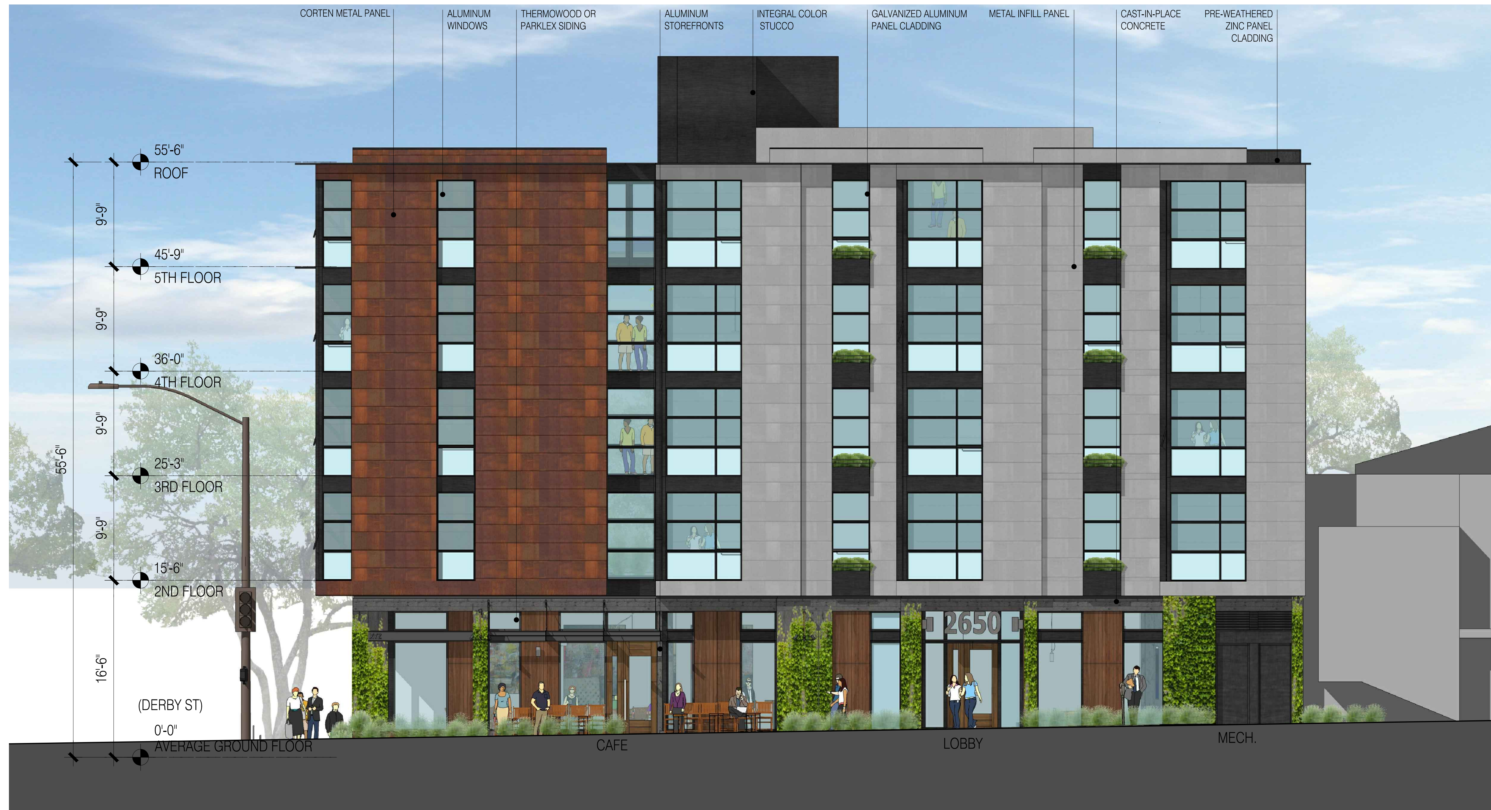
CORTEN METAL PANELS GALVANIZED ALUMINUM PANEL CLADDING PRE-WEATHERED ZINC PANEL CLADDING CAST-IN-PLACE CONCRETE METAL INFILL PANELS THERMOWOOD OR PARKLEX SIDING
