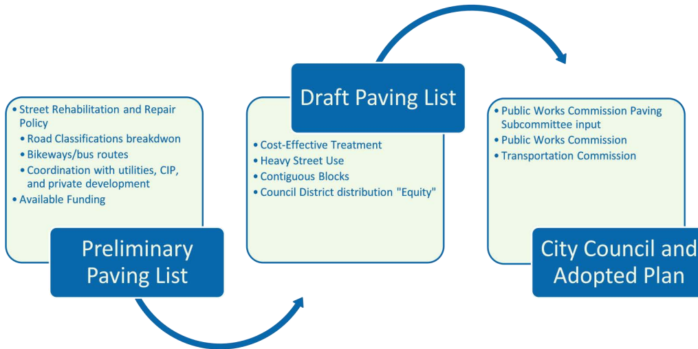
Figure 12. Process for Updating the Five-Year Paving Plan
