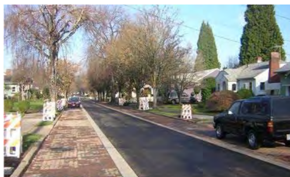
Permeable unit pavers have slight gaps which allow for surface water percolation. While this pavement type would be an additional source of groundbourne noise, the noise would be similar to that created by vehicles driving over asphalt.
