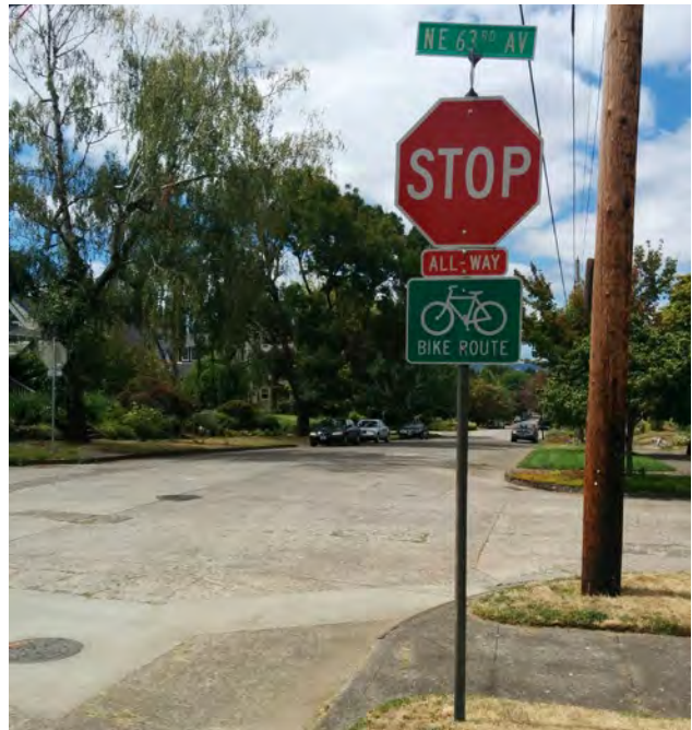
Typical stop sign placement, with R1-3P supplemental placard and stop bars on each leg of the intersection.
