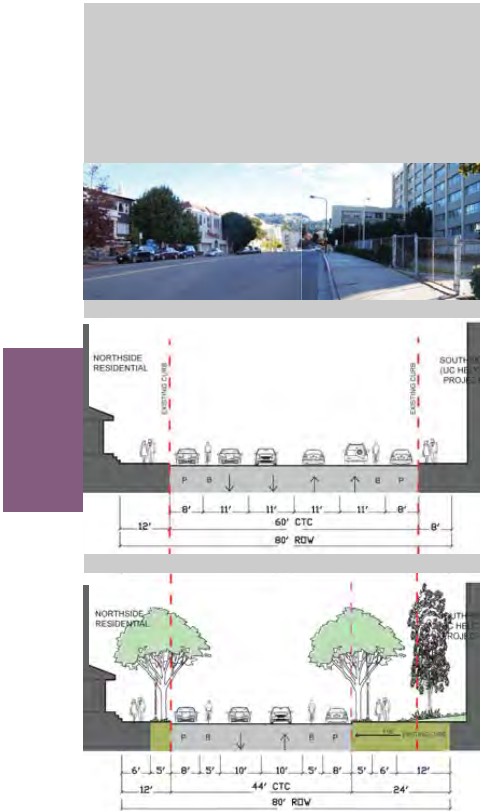
Figure d.33. Hearst Avenue / Ohlone Greenway (Shattuck to Oxford). Analysis suggests that traffic lanes can be eliminated, so that this dimension can be reallocated to bicycle lanes and a landscaped greenway.
