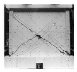
Similar test results have been found by Barda (1976) and Hidalgo (2002). Currently ASCE 41 acceptance limits and modeling guidelines for such walls allow deformation limits higher than shown in testing. These guidelines recommend more conservative limits. In older concrete wall buildings, horizontal reinforcement ratio is typically close to minimum reinforcement requirements of 0.0025, and thus such walls can suffer rapid strength loss soon after the onset of diagonal cracking.
