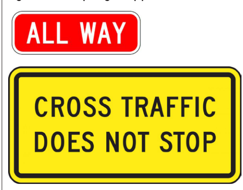
Figure 10: Stop Sign Supplemental Placards
