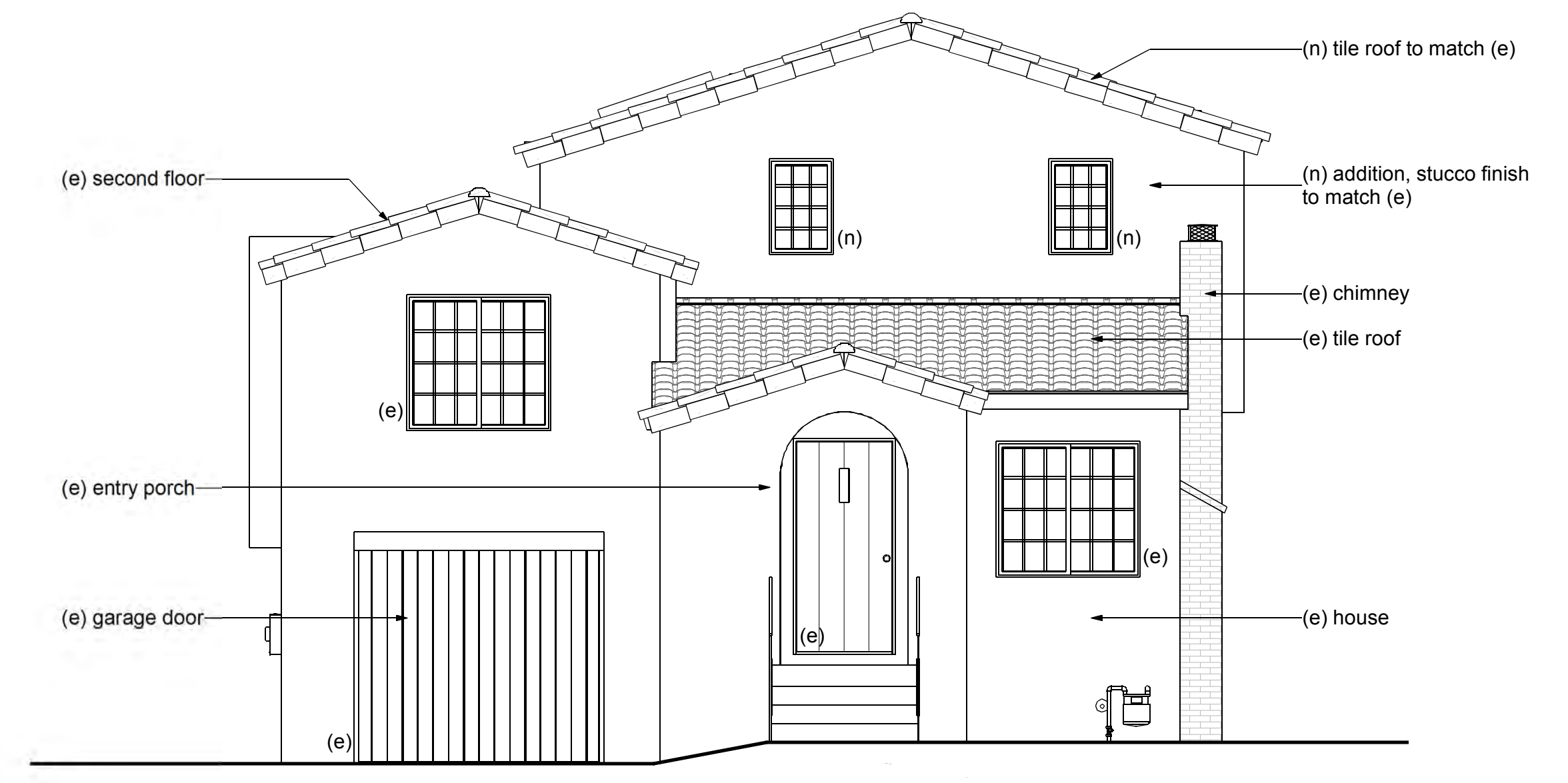
1 Proposed North Elevation - Front AUP Modification
