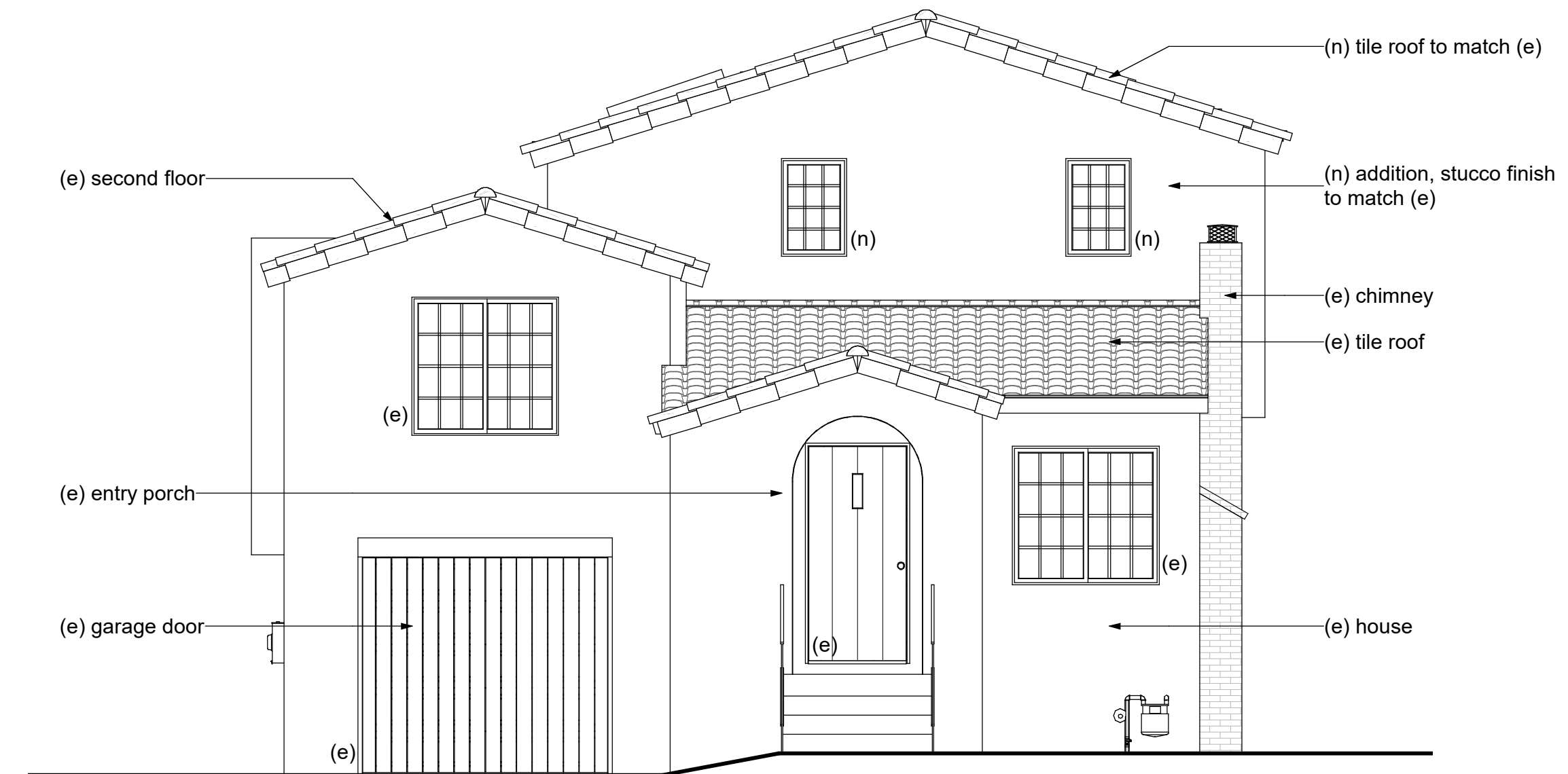
1 Proposed North Elevation - Front Original Approved AUP
