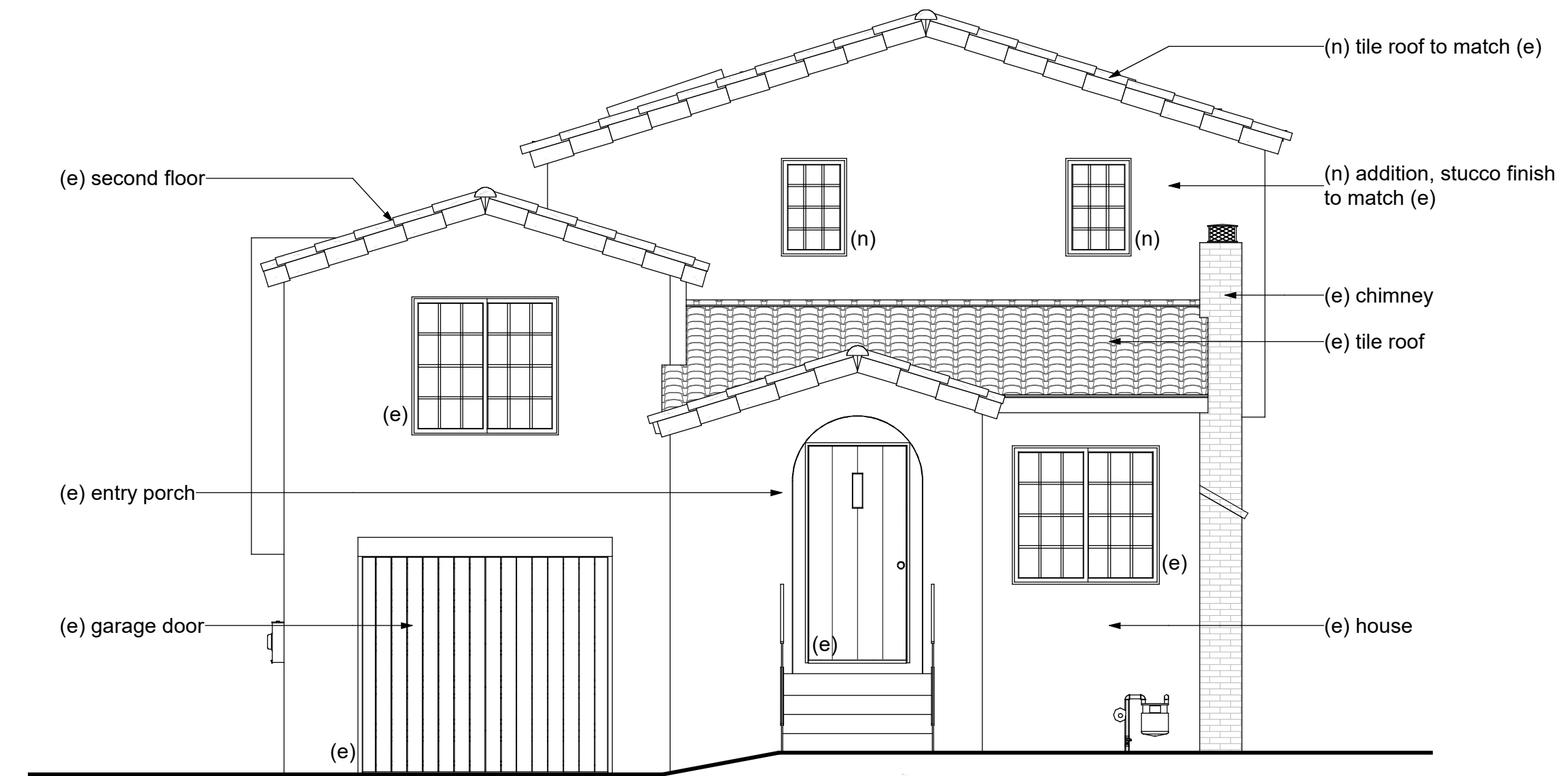
1 Proposed North Elevation - Front Original Approved AUP
