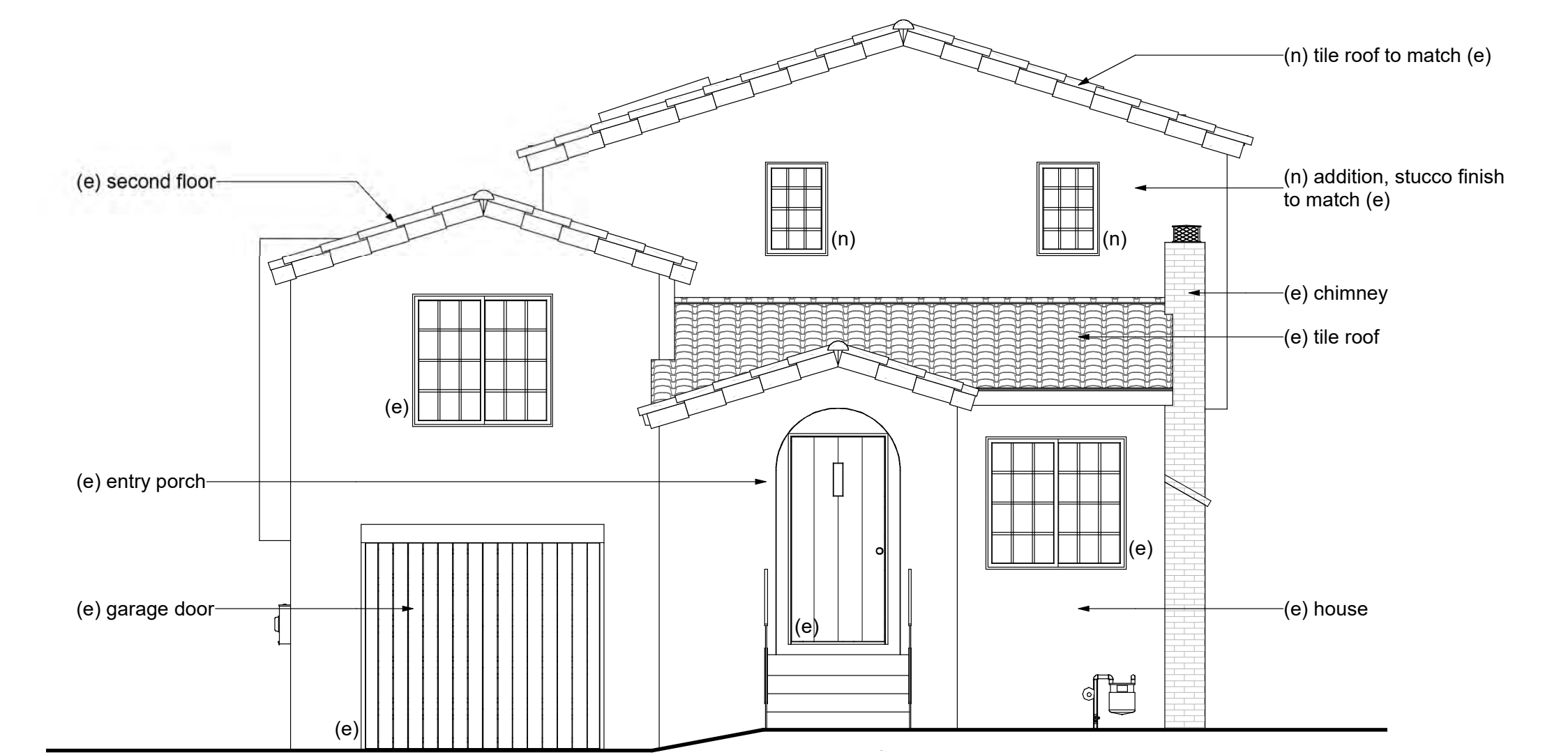
1 Proposed North Elevation - Front AUP Modification
