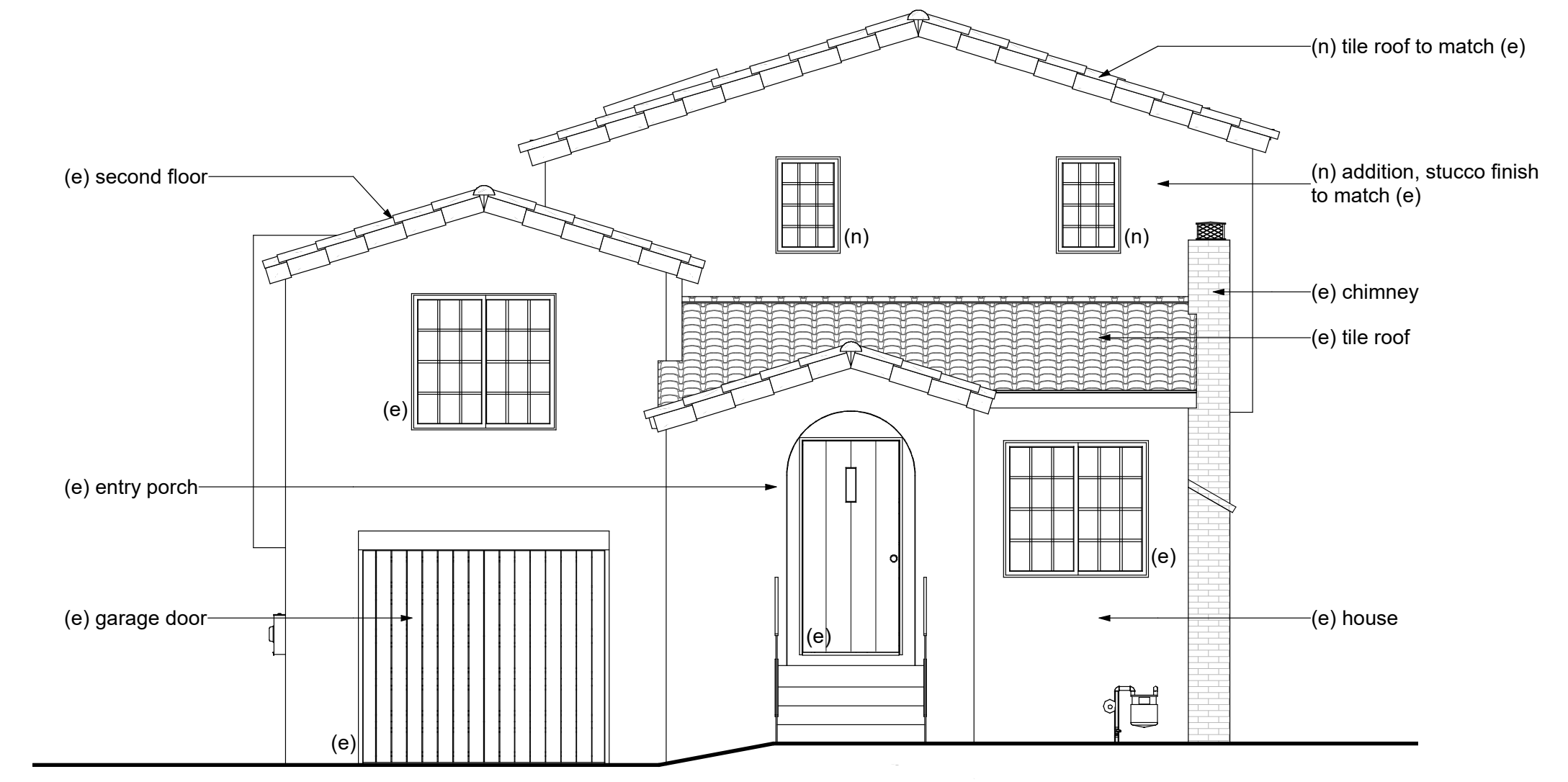
1 Proposed North Elevation - Front Original Approved AUP
