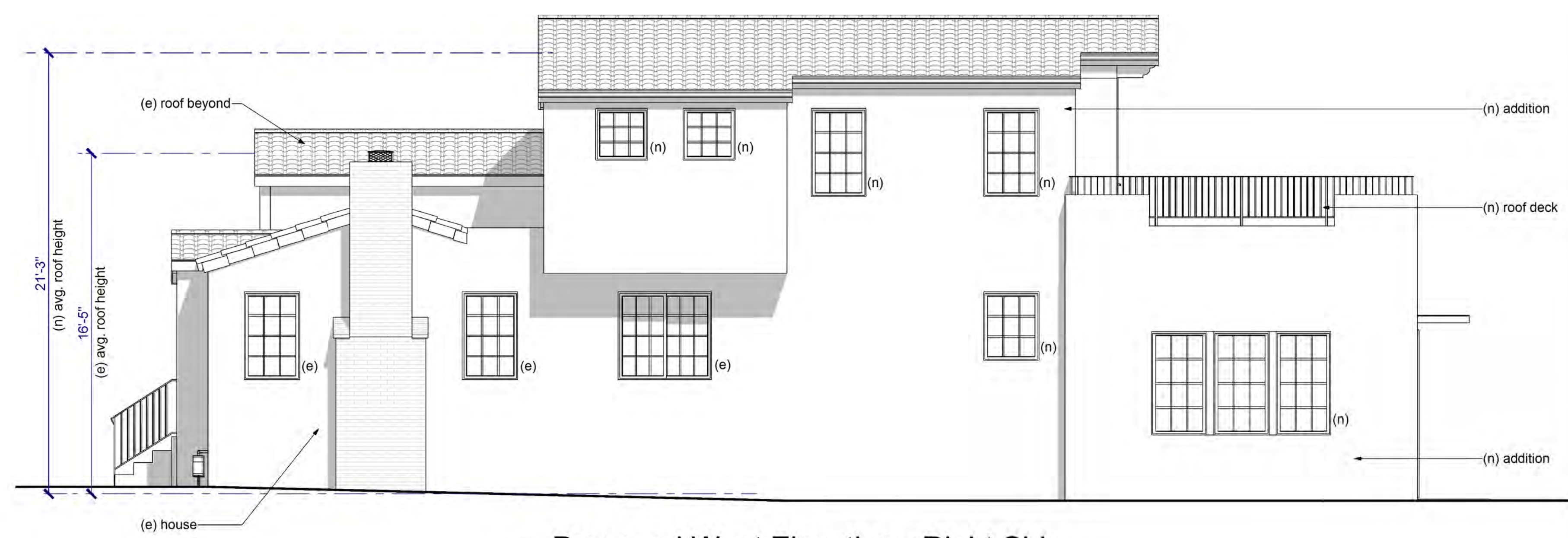
3 Proposed West Elevation - Right Side AUP Modification
