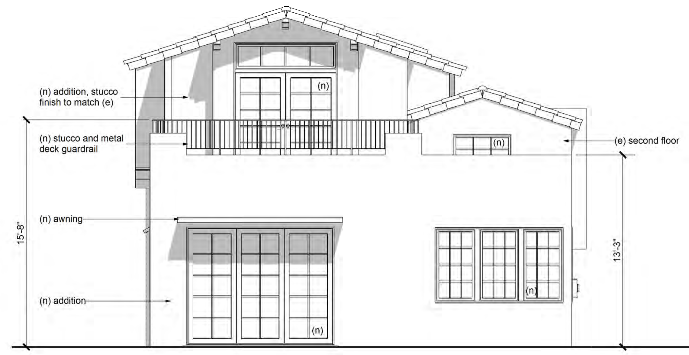
4 Proposed South Elevation - Rear AUP Modification
