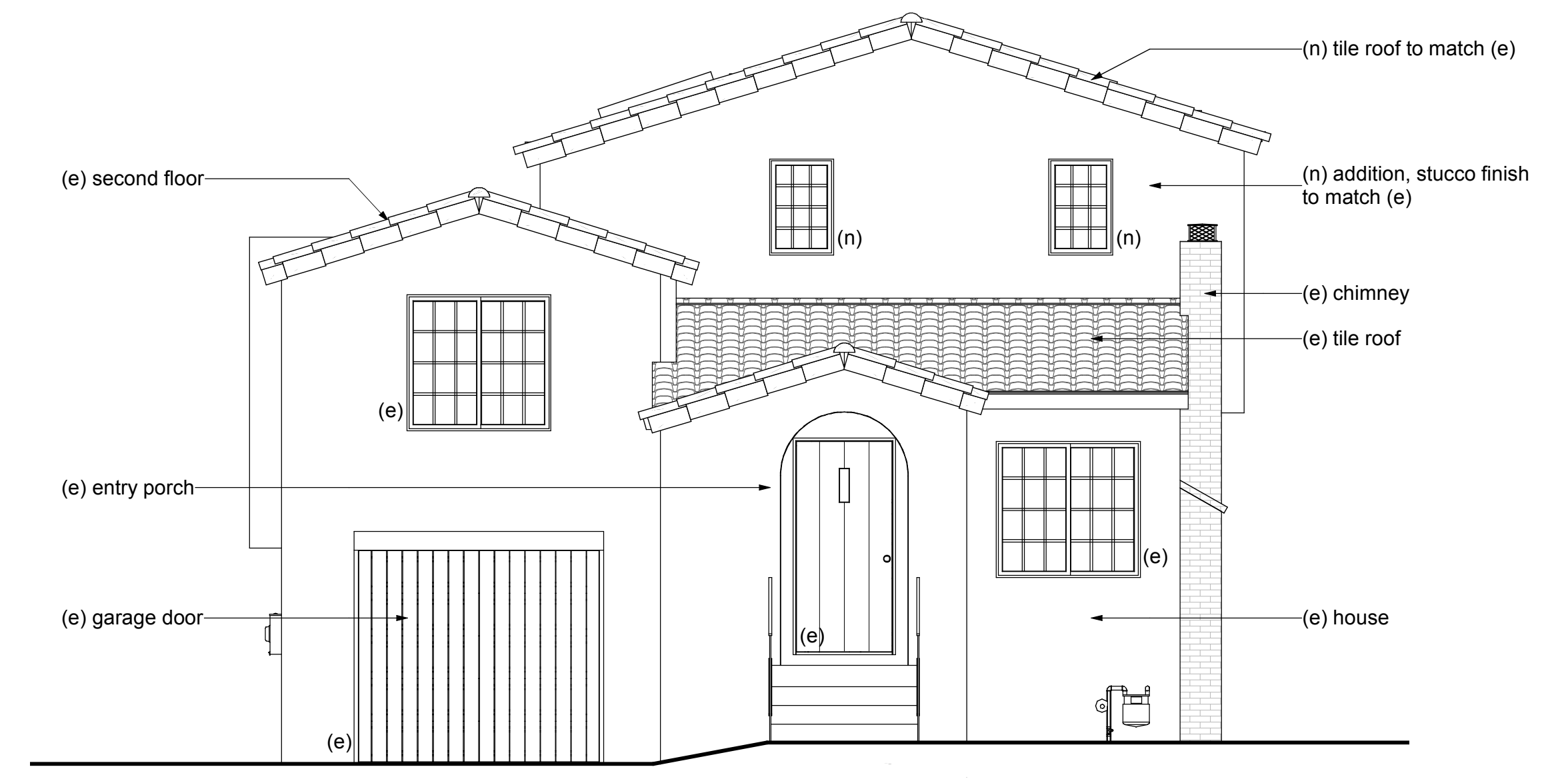
1 Proposed North Elevation - Front AUP Modification
