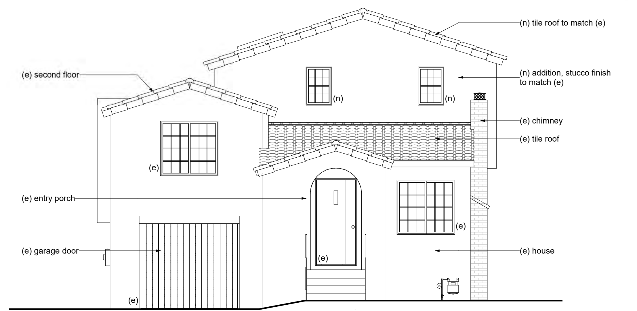
1 Proposed North Elevation - Front AUP Modification
