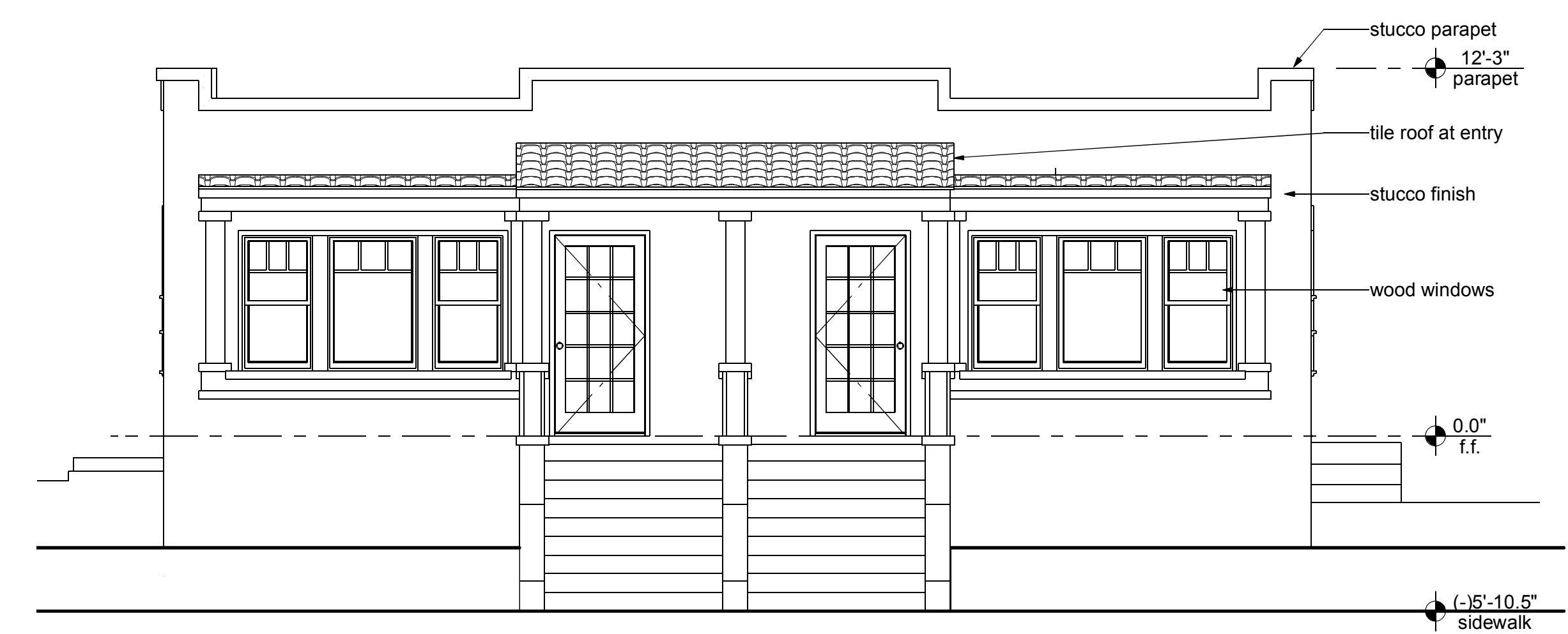
2 Existing West Elevation - Front
