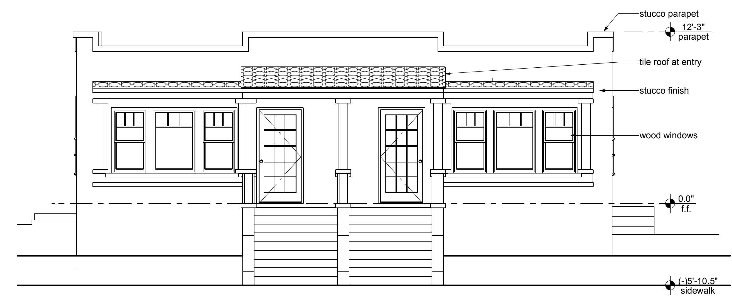
2 Existing West Elevation - Front
