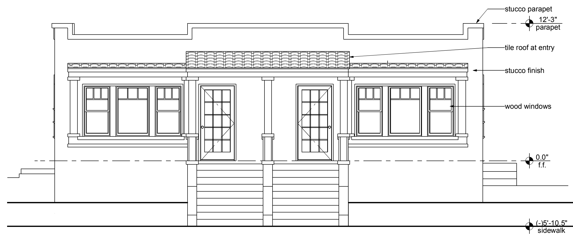
2 Existing West Elevation - Front
