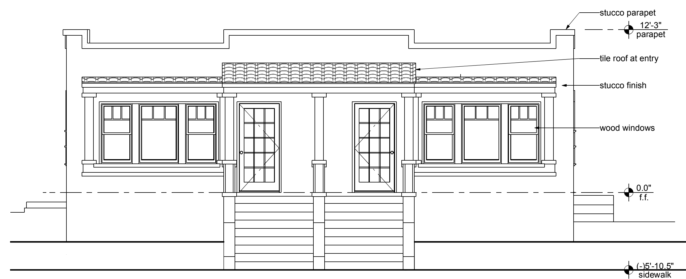
2 Existing West Elevation - Front
