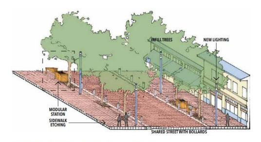
Ultimate Condition. TRPR proposes a plaza-like shared street and new lighting as a final phase. Sidewalk etching may remain or, if necessary, sidewalks can be replaced.
