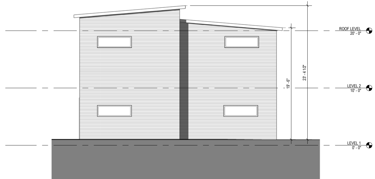
1 DAFFODIL & EDELWEISS EAST ELEVATION 1/8" = 1'-0"
