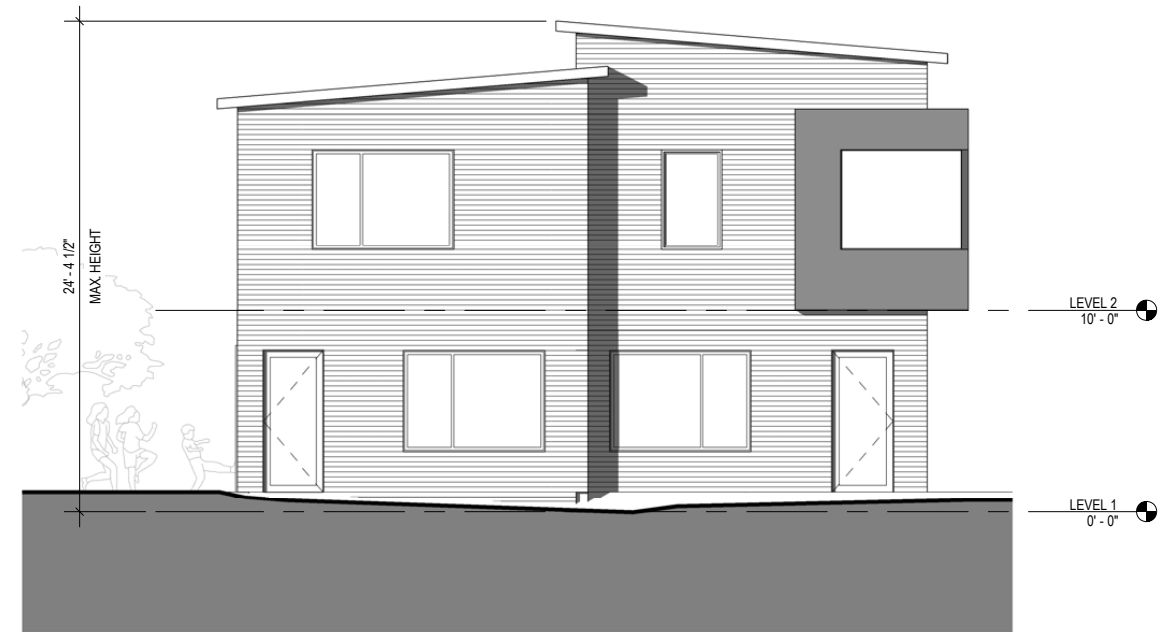
1 DAFFODIL & EDELWEISS WEST ELEVATION 1/8" = 1'-0"
