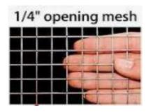
• Bury hardware cloth 12" (inch) into the ground all the way around the coop and run to deter burrowing from underneath.
